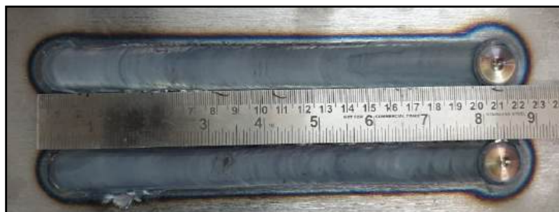
Fig. 1: Defect free EN-24 (AISI 4340) steel FSPed sample of total length 400 mm and depth of 4mm developed by using WC6%Co tool
