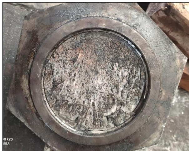
Fig: Failed tie Rod of Crop Shear Key words: Crop Shear Tie Rod, Brittle Fracture
