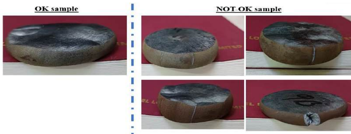
Fig. 1: Evidence of OK(Zero Rating) & NOT OK(01 & 02 Rating) Sample.
