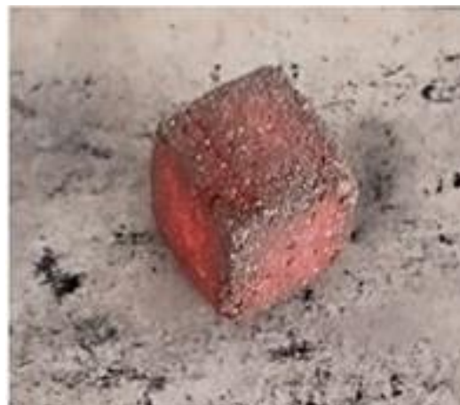
Fig.-1 RC-6 (One of the Thermal Spalling Results)
